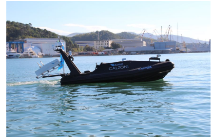
(c) Fast unmanned surface vehicle equipped with unmanned rescue capsule
