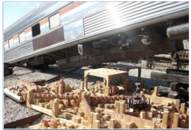
Fig. 1: Robot navigating through a standardized step-field at the test-site of the Center for Robot-Assisted Search and Rescue (CRASAR)[6]
