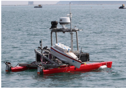
(a) Unmanned surface vehicle for victim rescue equipped with unmanned rescue capsule
