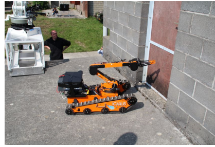
(b) Small UGV opening the door after being deployed by the large UGV on the first floor
