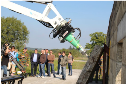
(a) Breaching through concrete walls blocking entrance to buildings
